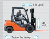
This system uses a switch sensor built into the operator's seat to detect the presence of the operator. If the operator is not in the normal operating position, travel power is interrupted and load handling operations are stopped.
