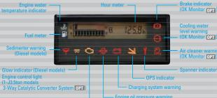
When the engine controller detects a malfunction such as high engine water temperature, this function automatically restricts engine output or stops the engine and informs the operator by the combination meters, to help prevent further
